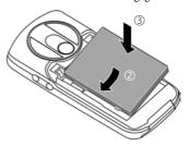
To remove, press the retaining tab on the side of the battery, then lift the battery out.  Place the battery cover on the phone slightly off centre
