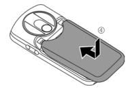
• To remove, press the battery cover ⑤, and slide it off the phone ⑥.
