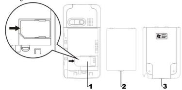
■ Installing the Battery
