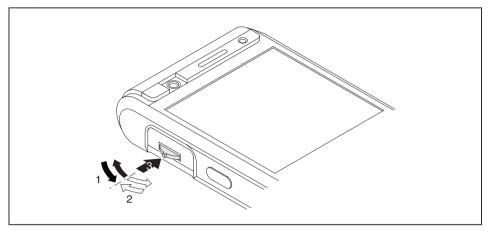
With the scroll button you can scroll up or down and forward or backward (1, 2) within the menu or application. You activate menu entries by pressing the middle scroll button (3).
