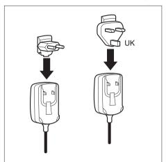
Push the matching mains adapter plug into the mains adapter in the direction of the arrow until it engages.
