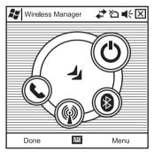
To activate or deactivate the telephone, Bluetooth or WiFi/WLAN, touch the corresponding WiFi, Bluetooth or Phone symbol.
