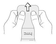
**3.** With your finger, lift up the back cover from the bottom side to remove it.
