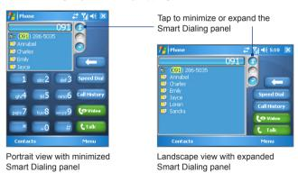
When you use the hardware keyboard to dial a number, the digits entered will be displayed on the right side of the entry box and the equivalent letters will appear on the left side. Whereas tapping the Phone keypad will display only the digits in the entry box.
