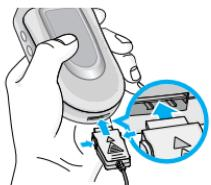
1. With the arrow facing you as shown in the diagram push the plug on the battery adapter into the socket on the bottom of the phone until it clicks into place.
