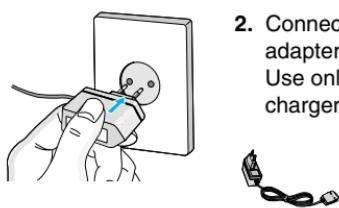
2. Connect the other end of the travel adapter to the mains socket. Use only the included packing charger.
