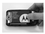
4 Pull the battery back towards the bottom part of the handset to ensure that the battery is in good contact with the handset.
