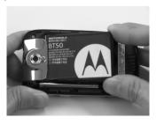
**3** Push the battery forward and then push it down until it totally falls into the battery compartment.
