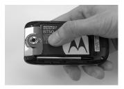
**5** Place the battery door on the phone and slide it up to lock shut.
