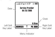
When  $\blacksquare$  is displayed, you can press  $\blacksquare$  to open the menu. Labels at the bottom corners of the display show the current soft key functions. Press the left or right soft key to perform the function indicated by the label. For soft key locations, see page 1.
