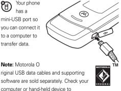
determine the type of cable you need. To **transfer data** between your phone and computer, you might need to install the software included with the Motorola Original data kit. See the data kit user's guide for more information. To make **data calls** through a connected computer, see page 72.
