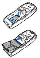
5. Align the top of the back cover with the top of the phone (1), press the bottom of the back cover to lock it (2).
