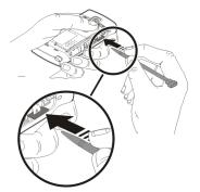
If the SIM card is not properly in place, the device can only be used in the offline profile.
