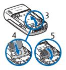
5. Swing the SIM card holder closed. The gold-colored contacts on the SIM card meet the gold-colored contacts on the inside of the phone.
