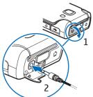
Do not connect products that create an output signal as this may cause damage to the device. Do not connect any voltage source to the Nokia AV connector.
