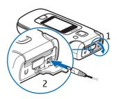
The charging time depends on the charger and the battery used. Charging a BL-5F battery with the AC-4 charger takes approximately 45 minutes.
