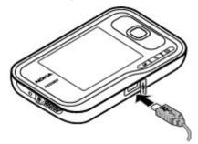
To avoid corrupting data, do not disconnect the USB data cable during data transfer.
