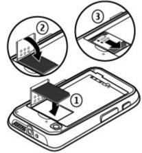
4. Align the battery contacts with the battery compartment connectors, and insert the battery.
