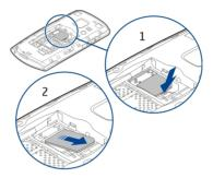
Press the release spring (1), and slide out the SIM card (2).
