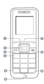
G 4-way navigation key In Idle mode, adjust the volume level (up/down) or user-defined menus (left/right): In Menu mode, scroll through menu options
