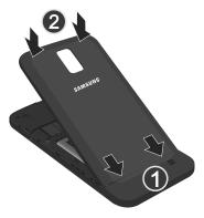
Press all along the edge of the back cover until you have a secure seal
