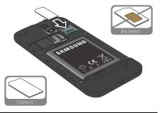
Note: If the card is not inserted correctly, the phone will not detect the SIM card. Re-orient the card back into the slot if the SIM is not detected.
