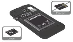
To remove, push on the memory card until it clicks and is released. Then grasp the memory card and remove it from the phone.
