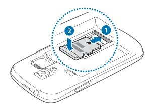
3 Push the memory card down into the slot and then slide it backwards until it locks into place.
