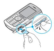
2. To remove the card, push it in and release so that it is disengaged from the slot. Then slide the card out.
