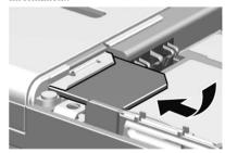
Remove the battery (if it is in place) and insert the SIM card into the SIM card holder. A PIN code is supplied with the SIM card and must be entered when switching on the phone for the first time
