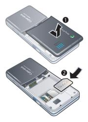
2 Slide the SIM card into its holder with the gold-coloured contacts facing down.
