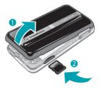
Remove the battery cover and insert the memory card with the goldcoloured contacts facing up.
