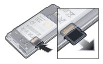
Remove the battery cover and press the edge of the memory card to release and remove it.
