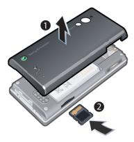
Remove the battery cover and insert the memory card with the goldcoloured contacts facing up.
