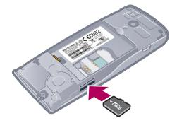
Remove the battery cover and insert the memory card with the gold-coloured contacts facing down.
