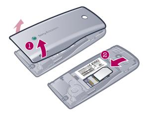
Open the cover and insert the SIM card with the gold-coloured contacts facing down.
