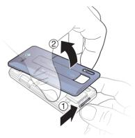
1 Slide and hold the clasp sideways and remove the battery cover.
