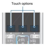
Select an action shown at the bottom of the screen by pressing the left, centre or right touch option.
