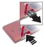
• Press the edge of the memory card to release and remove it.
