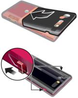
2 Slide the battery cover into place and lock it.
