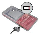
1 Connect the charger to the phone. It takes approximately 2.5 hours to fully charge the battery. Press a key to view the screen.
