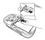
Press the edge of the SIM card to release it from the slot
