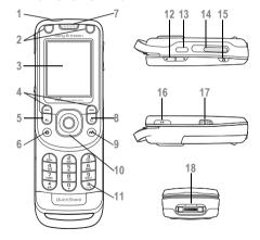
Power on/off button Game A and game B buttons Screen Selection keys 5 Back key Internet button Ear speaker 8 Clear key 9 WALKMAN<sup>TM</sup> key 10 Navigation key #= Silent key 11 12 Volume, camera and picture zoom buttons 13 Infrared port 14 External speaker 15 Camera button Play/Pause button 16 17 ► Some Lock switch → 70 Keypad lock 18 Stereo headset and charger connector
