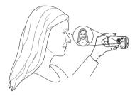
Hold the phone as shown in the illustration, so that you can see your reflection in the mirror next to the lens. Press the camera button to take the picture.
