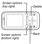
Switch camera/video (5) or (9) Adjust brightness (6) or (6)
