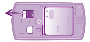
• Remove the battery cover, then draw the memory card outwards to remove it.
