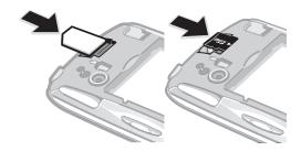
Remove the battery cover, then insert the SIM card and the memory card in the relevant slots.
