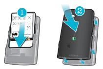
Insert the battery with the battery usage labels facing down and the connectors facing each other.
