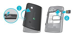
Slide in the SIM card and the memory card with the gold-coloured contacts facing down.
