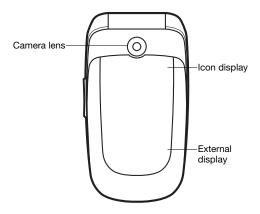
The icon display lights up when the phone is in silent mode and shows information about new events and battery charging. The external display shows information such as time. Press a volume button to activate the external display.
