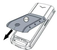
> Turn the locking screw (02) a quarter of a turn anticlockwise, gently pivot (by no more than 45 degrees) and lift off the back cover (03) towards you as shown. If you accidentally remove the back cover while the phone is switched on, the phone will automatically switch off.
