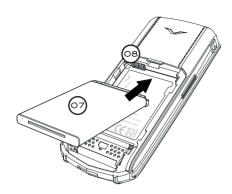
Insert the battery (07) top end first. Ensure that the contacts on the top end of the battery align with the contact points (08) inside the battery compartment.
