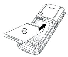
Insert the battery (01) top end first. Ensure that the contacts on the top end of the battery align with the contact points (02) inside the battery compartment.
