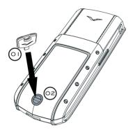
With the back of your Vertu phone facing you, position the back cover release key (01) very carefully into the slot of the locking screw (02). Ensure the key does not slip out of the slot.
