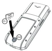
With the back of your Vertu phone facing you, position the back cover release key (01) very carefully into the slot of the locking screw (02). Ensure the key does not slip out of the slot.
