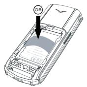
If you do not re-insert the battery or insert another battery right away, insert the plastic placeholder (05) originally supplied with your Vertu phone before replacing the cover.
