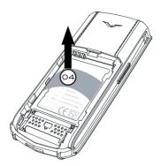
> Remove the plastic placeholder (04) from your Vertu phone before inserting the battery.
