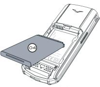
> Gently pivot the battery (04) from the bottom and lift it upwards and outwards from your Vertu phone.
