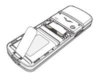
> Ensure that the battery is seated correctly before replacing the back cover.
