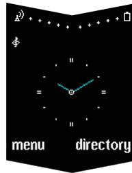
The battery charge and signal strength indicators appear at the top of the display.
