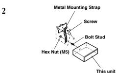
When your vehicle has the Bracket, mount the long hex bolt onto the rear panel of the CDE-9873RB/CDE-9871R/CDE-9871RR and put the Rubber Cap on the hex bolt. If your vehicle does not have the Mounting Support, reinforce the head unit with the metal mounting strap (not supplied). Connect all other leads of the CDE-9873RB/CDE-9871R/CDE-9871RR according to details described in the CONNECTIONS section.
