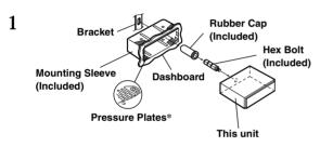
\* If the installed mounting sleeve is loose in the dashboard, the pressure plates may be bent slightly to remedy the problem.
