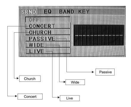
**Note:** This function only is used with the remote control in CD/MP3/USB/SD mode. Once you have one of these settings on. You will no longer have Bass & Treble adjustments until this feature is set to off.
