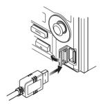
**2** Connect the USB device to the unit using the supplied cable.
