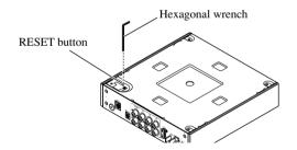
**3. Replace the cover to assure the reset button is not accidentally pressed.** The cover may be attached vertically or horizontally.
