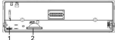
Pressing RESET hole will erase the clock setting and stored stations.
