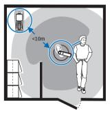
picture. The connection is subject to interference from distance and obstructions (shown in light grey) or other electronic devices.
