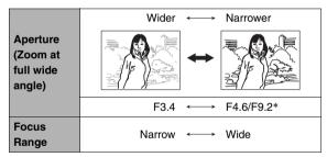
\* The camera has a built-in ND filter to limit exposure. F9.2 is the aperture when the ND filter is being used.
