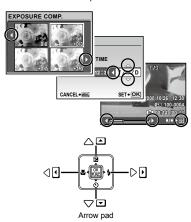
Operation guides displayed at the bottom of the screen indicate that the **MENU** button, B button, zoom buttons, or h button be used.
