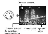
2 After pressing <sup>(2)</sup>, select the aperture value / shutter speed using <sup>(2)</sup> (3) (3) (3), and pressing the (3) button.
