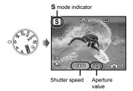
2 After pressing (2), select the shutter speed using (2)(3), and pressing the (2) button.
