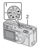
The Night Portrait mode combines the electronic flash with a "slow shutter" mode. This unique feature allows you to photograph close subjects against the natural night background. Since the shutter speed is slow, we highly recommend using a tripod to steady the camera.
