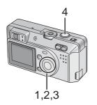
In some situations the illumination of the background and your subject may differ. Auto exposure systems may not always calculate the exposure correctly. This is a normal situation. This feature allows you to manually compensate the exposure.
