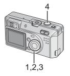
Pressing the shutter button once, the camera will automatically take 3 pictures changing exposure according to the set exposure compensation value.
