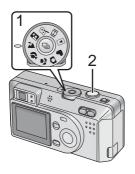
In Landscape mode the camera is adjusted to produce the greatest depth of field. This mode works best outdoors under direct sunlight at distances exceeding 32.8 feet (10 m).
