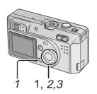
After taking a picture, the Auto review (P71) feature will cause the captured picture to be displayed on the LCD monitor for the designated time - 1 or 3 seconds. You may also check the picture using the method described below.
