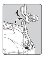
Pass the other end of the strap through the other strap lug on the camera, then secure it on the inside of the clasp.
