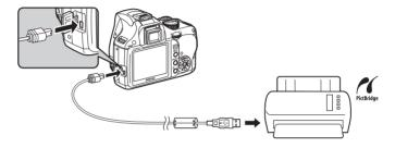
Connect the other end of the USB cable to a PictBridgecompatible printer.
