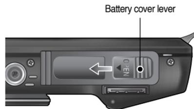
※ To open the battery chamber cover, slide it in the direction shown above.
