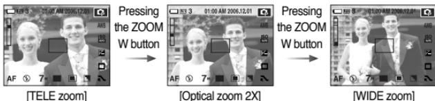
Digital zoom WIDE : When the digital zoom is in operation, pressing the ZOOM W button will reduce the digital zooming in steps. Releasing the ZOOM W button stops digital zooming. Pressing the ZOOM W button will reduce the digital zoom and then it will continue to reduce the optical zoom until the minimum setting is reached.
