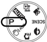
Selecting the program mode will configure the camera with optimal settings. You can still manually configure all functions except the aperture value and shutter speed.
