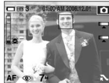
3. Press the shutter button halfway. The focus frame turns to green when the focus is activated.
