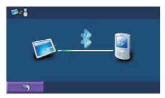
put the mobile phone near the PND, and let your mobile phone search the GPS device to pair, when mobile phone detect the GPS device, the pin code will be asked to enter, and the default pin code is 8888, when it shows succeeed, the connection is established; when it shows failed, the connection is not established.
