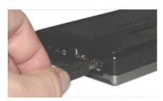
→ Use the plug to insert the mains section in the socket.
